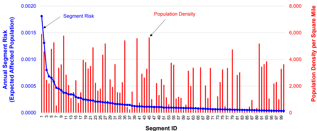
FIGURE 5 Segment risk and population density distributions (the risk is ranked in a descending order; the top 100 segments are displayed)
