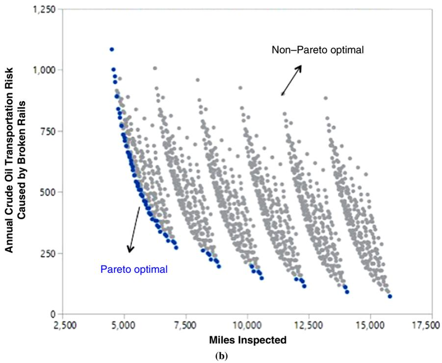
FIGURE 2 Pareto optimization of crude oil transportation risk caused by broken rails, by total miles to inspect: (a) three categories of segment risk, all with the same inspection frequency, and (b) four categories of segment risk, all with the same inspection frequency.
