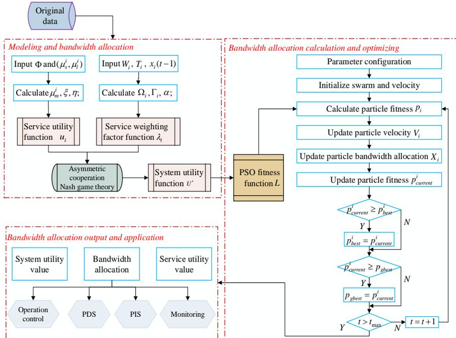
Fig.3. Bandwidth allocation scheme based on N-PSO
