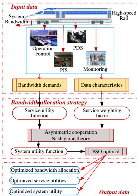
Fig.1. Overall scheme of high-speed TGCS bandwidth allocation
