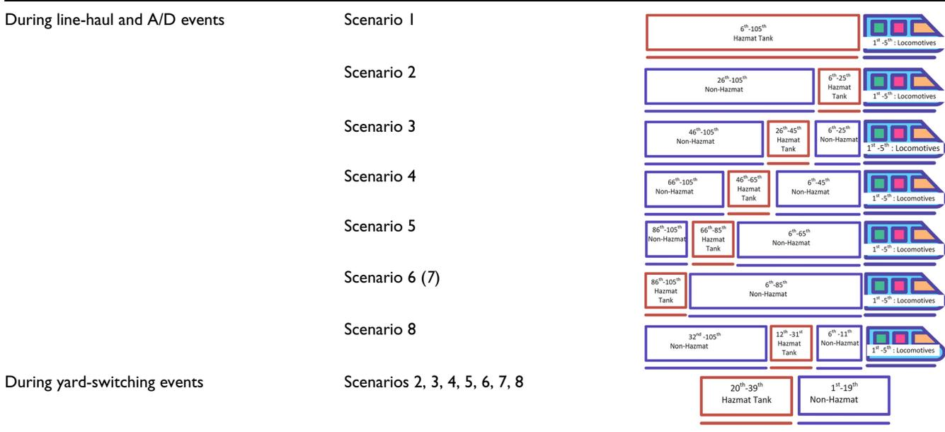
**Figure 4.** Train consists for each scenario during line-haul events, A/D events, and yard-switching events. Note: A/D = arrival/departure.
