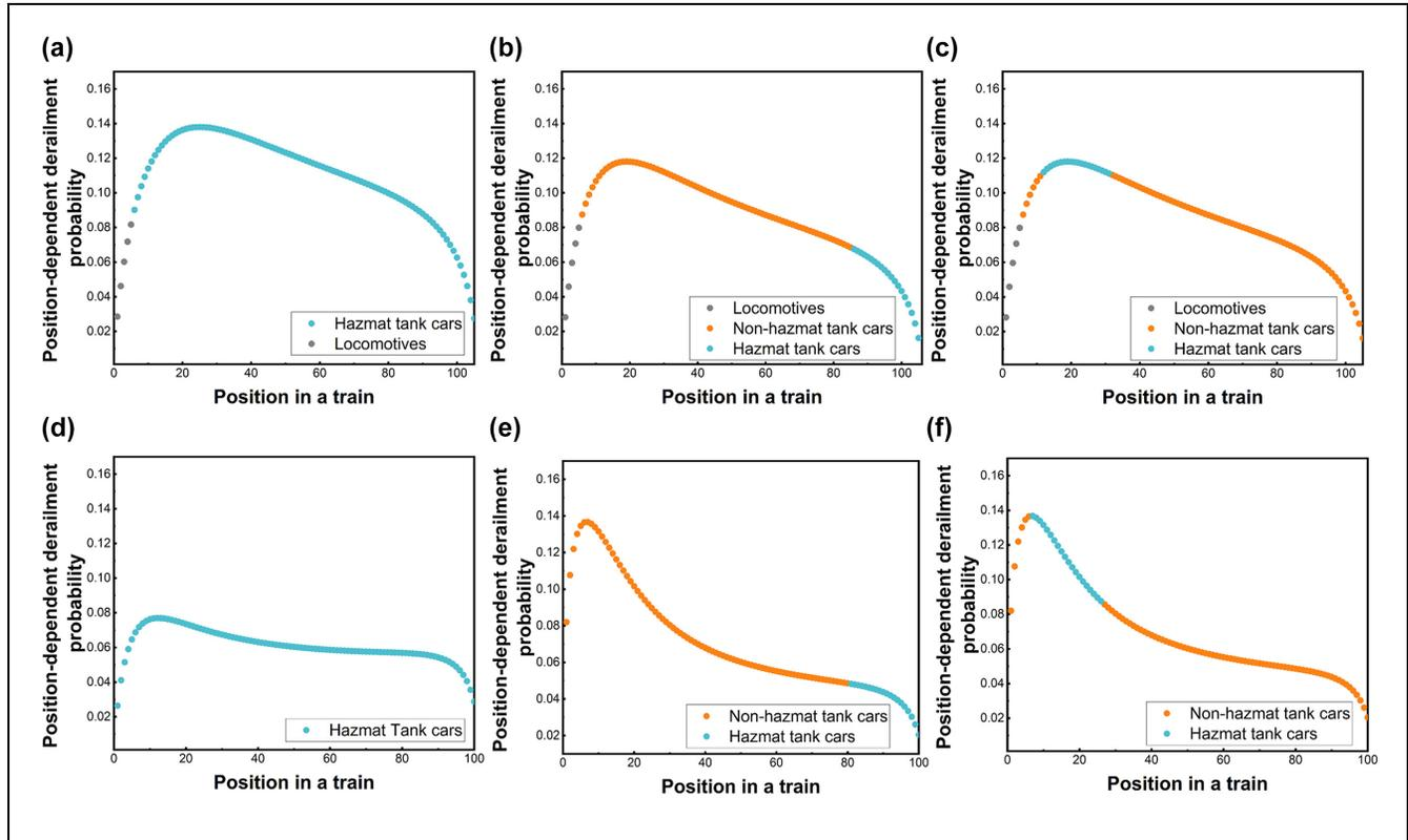
**Figure 3.** Position-dependent derailment probability during line-haul events and A/D events: (a) unit train, incidents on mainlines, Scenario 1; (b) manifest train, incidents on mainlines, Scenario 7 (or Scenario 6); (c) manifest train, incidents on mainlines, Scenario 8; (d) unit train, A/D incidents in terminals, Scenario 1; (e) manifest train, A/D incidents in yards, Scenario 7 (or Scenario 6); and (f) manifest train, A/D incidents in yards, Scenario 8.
