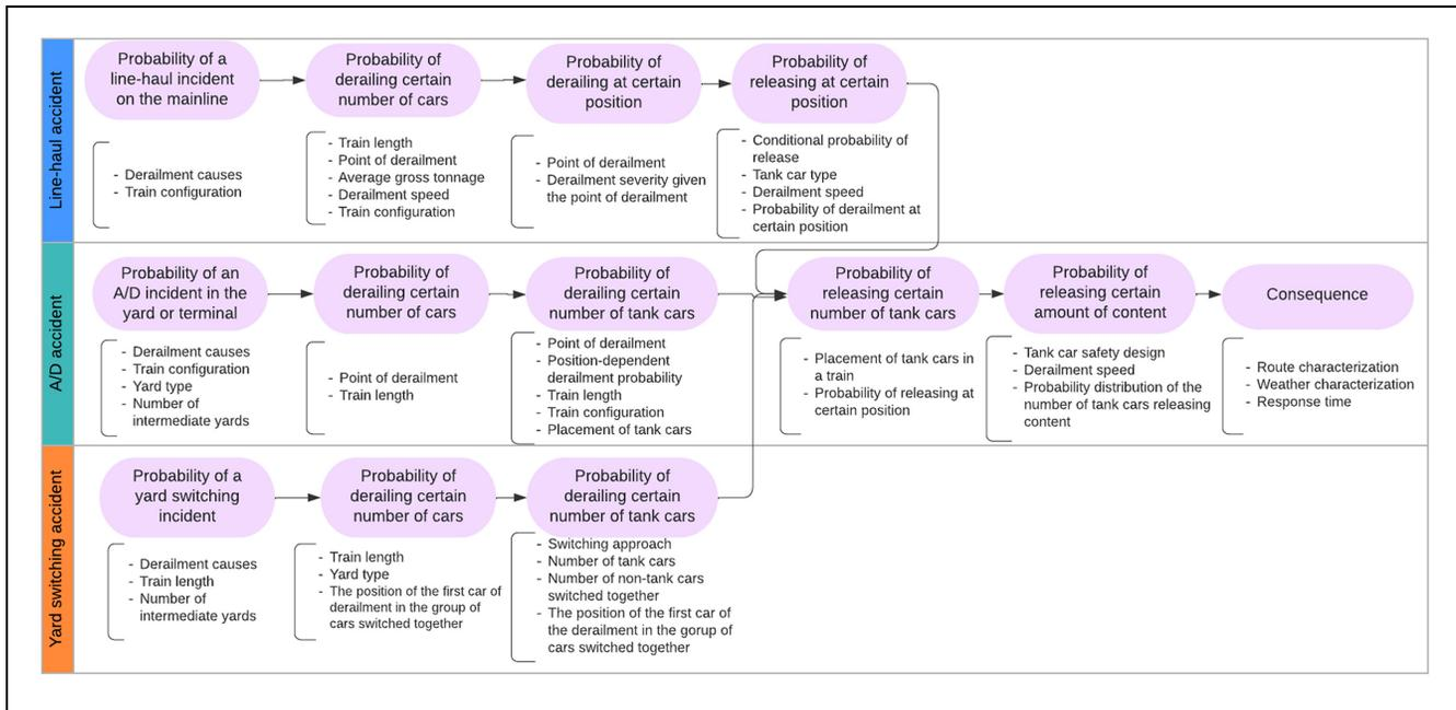
**Figure 1.** Flow chart of the event chains for different types of accident and the corresponding influencing factors (9).
