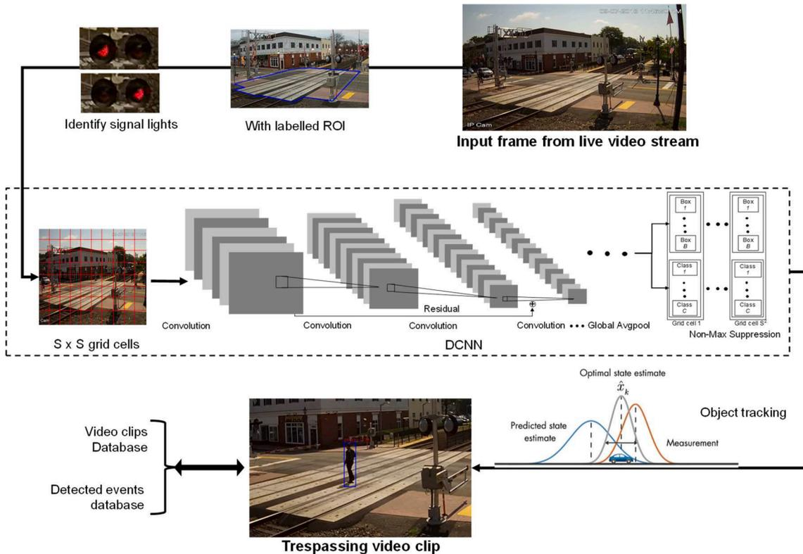
Fig. 5. Conceptual Trespassing Detection System Using Artificial Intelligence.
