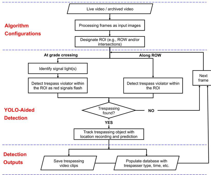
Fig. 3. General YOLO-Based AI Framework for Railroad Trespass Detection.
