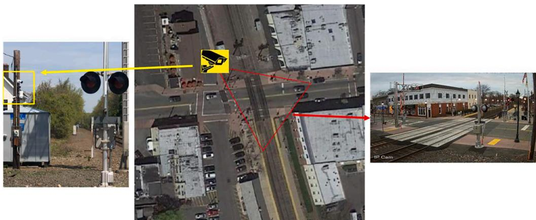
Fig. 7. IP Camera Placement at Selected Location.
