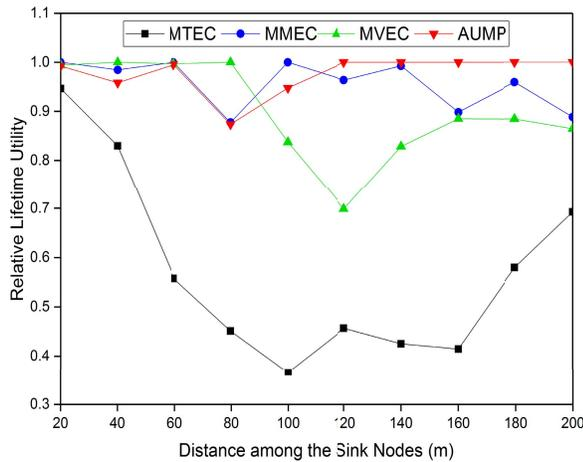
Fig. 7. Relative Lifetime Utility of MTEC, MMEC, MVEC and AUMP Protocols for Different Distances among Sink Nodes (Scenario 1).
