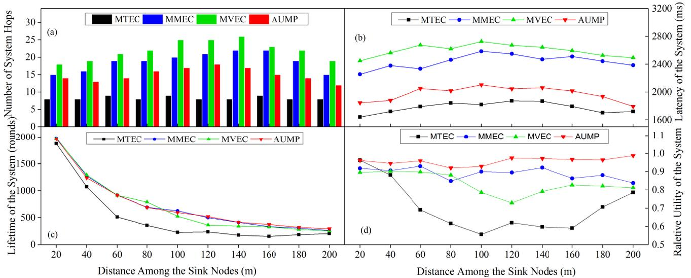
Fig. 6. The Performances of MTEC, MMEC, MVEC and AUMP Protocols for Different Distances among Sink Nodes (Scenario 1). (a) Number of Hops, (b) System Latency, (c) System Lifetime and (d) the System Relative Utility.
