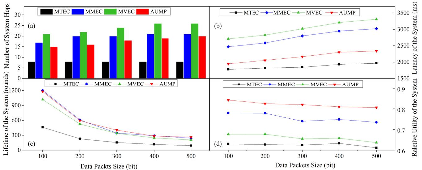
Fig. 14. The Performances of MTEC, MMEC, MVEC and AUMP Protocols for Different Data Packet Sizes (Scenario 3). (a) Number of Hops, (b) System Latency, (c) System Lifetime and (d) the System Relative Utility.
