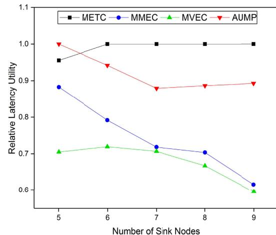
Fig. 10. Relative Latency Utility of MTEC, MMEC, MVEC and AUMP Protocols for Different Distances among Sink Nodes (Scenario 2).
