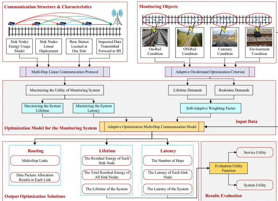
Fig. 1. Overall Scheme of the Adaptive Multi-Hop Communication Protocol for Railway Monitoring System.
