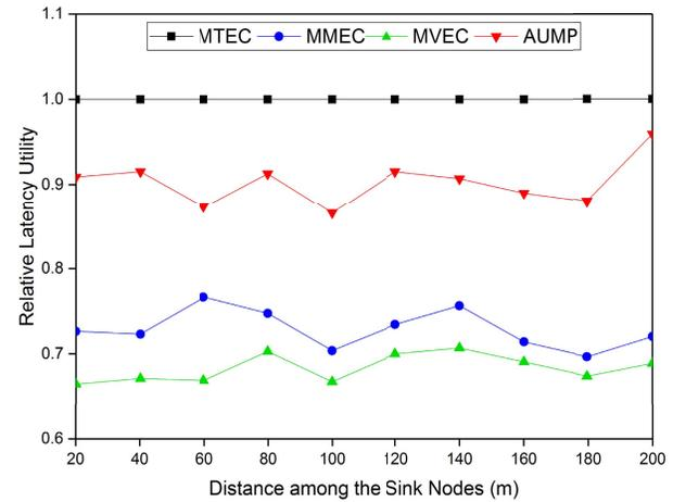
Fig. 8. Relative Latency Utility of MTEC, MMEC, MVEC and AUMP Protocols for Different Distances among Sink Nodes (Scenario 1).
