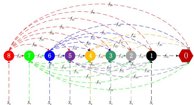
Fig. 5. Optimization Solutions of MTEC, MMEC, MVEC and AUMP Protocols ( $N = 8, S = 200$  bit,  $d = 20$  m).
