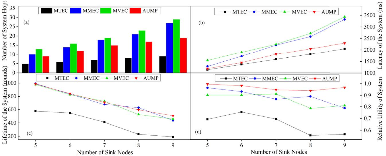
Fig. 11. The Performances of MTEC, MMEC, MVEC and AUMP Protocols for Different Number of Sink Nodes (Scenario 2). (a) Number of Hops, (b) System Latency, (c) System Lifetime and (d) the System Relative Utility.
