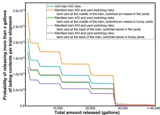
Fig. 17. The reverse cumulative distribution of the amount released per shipment in terminals (unit train) or in yards (manifest train).
