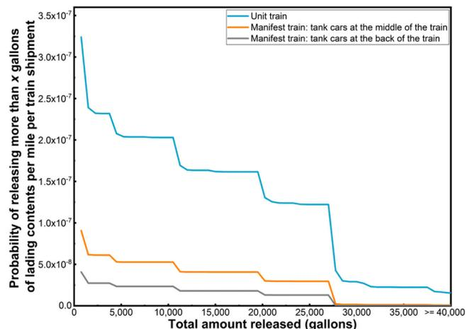
Fig. 16. The reverse cumulative distribution of the amount released per mile per shipment on the mainline segment.
