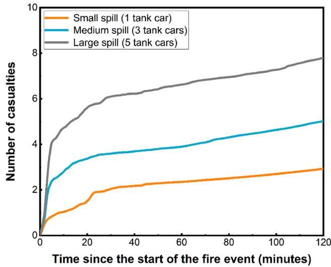
Fig. 5. Casualties from fire spread in the QUIC-FST analyses.
