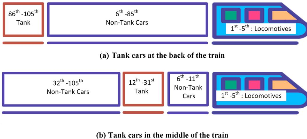
Fig. 8. Train consists of the five manifest trains (a) tank cars at the back of the train (scenarios 2 and 3), and (b) tank cars in the middle of the train (scenarios 4 and 5).
