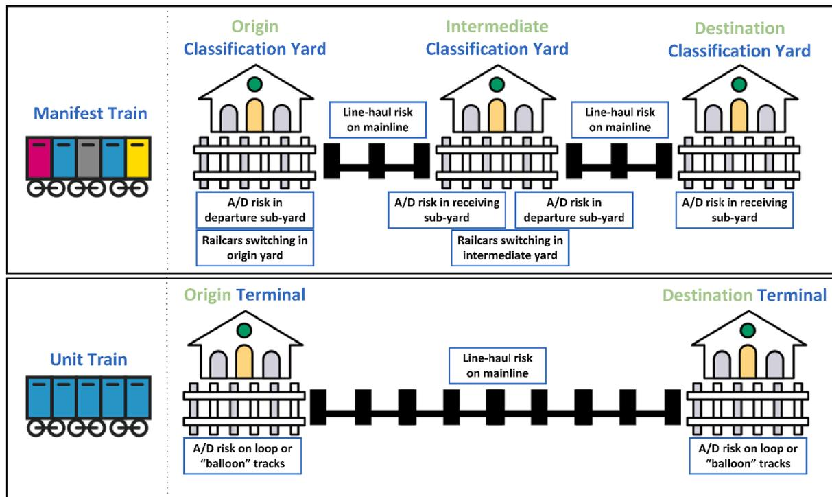
Fig. 1. Types of risks encountered by different train configurations.
