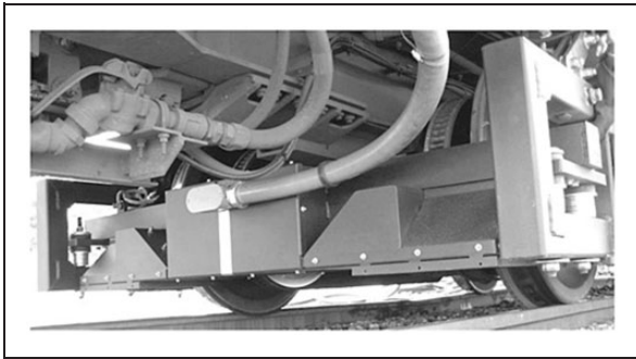
Figure 2. Autonomous Track Geometry Measurement System Technology (ProgressiveRailroading.com/railproducts, 2016).
