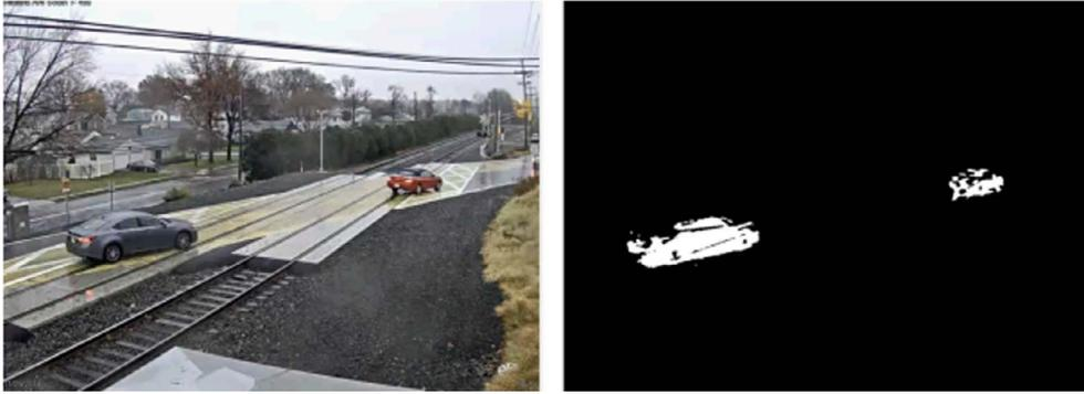
Fig. 8. Moving-Objects Mask in Rain.
