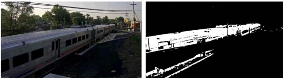
Fig. 9. Mask corresponding to a frame containing the train.
