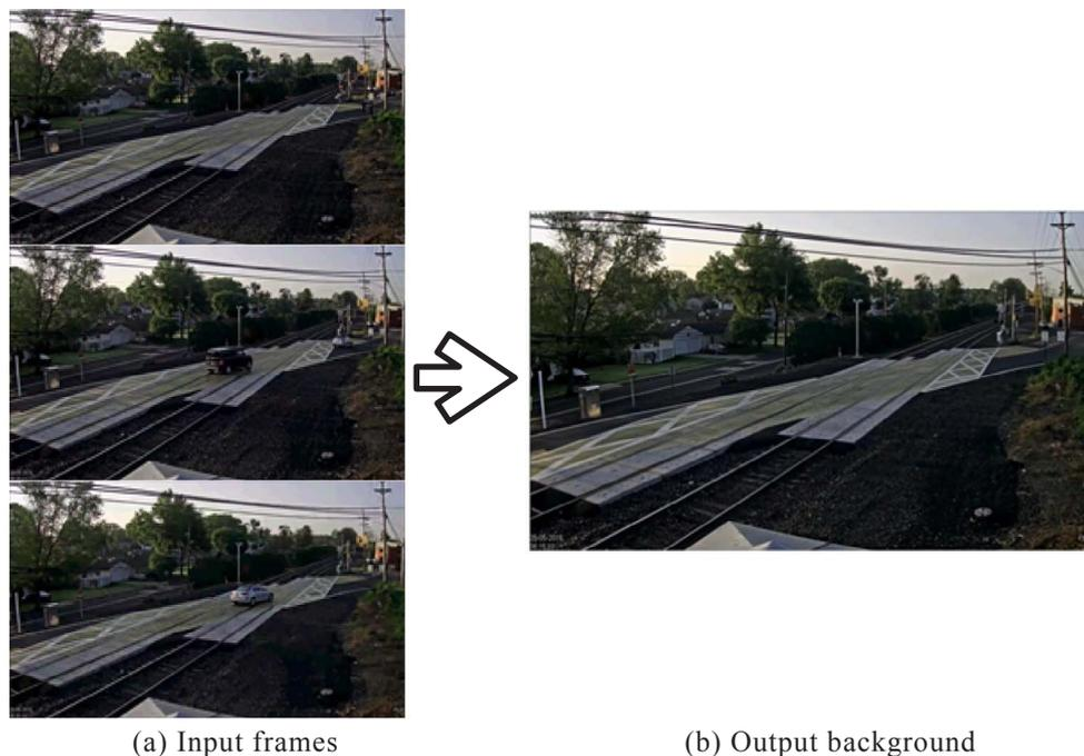
Fig. 5. Background learning (a) input frames to determine (b) output background.
