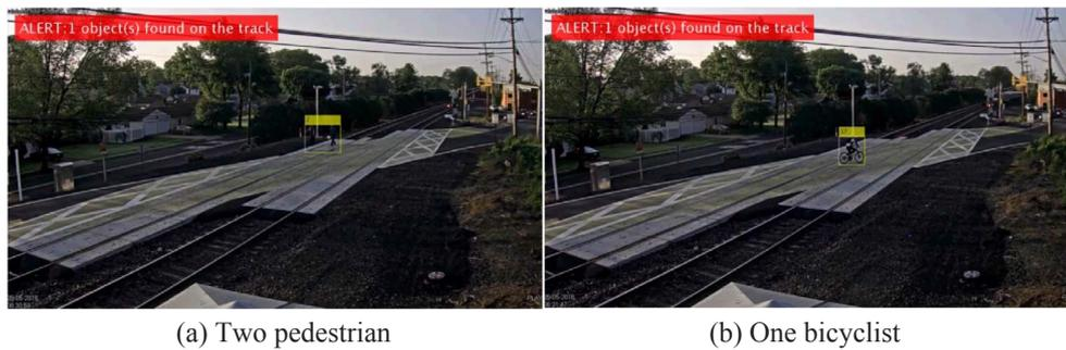
Fig. 10. Two trespassing near-miss events detected by the AI algorithm: (a) two pedestrians and (b) one bicyclist.
