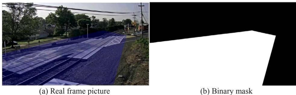
Fig. 2. Region of Interest (ROI) as indicated by (a) the blue polygonal area on the tracks, and (b) binary polygon mask.
