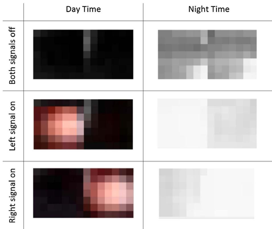
Fig. 4. Intensity difference of stop signal during day and night.
