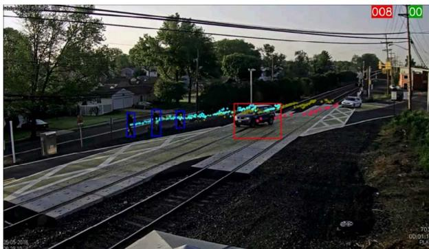
Fig. 11. Traffic counting with bounding boxes and tracking.
