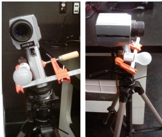
Fig. 4. Luminance meter and light source (left: front view; right: side view).
