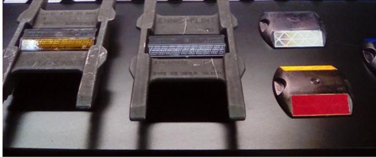
Fig. 1. Examples of RPM samples.
