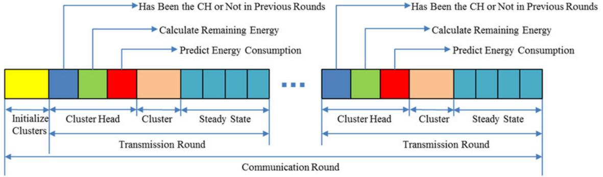
Fig. 3. Structure of the communication round of the proposed CVLMP.
