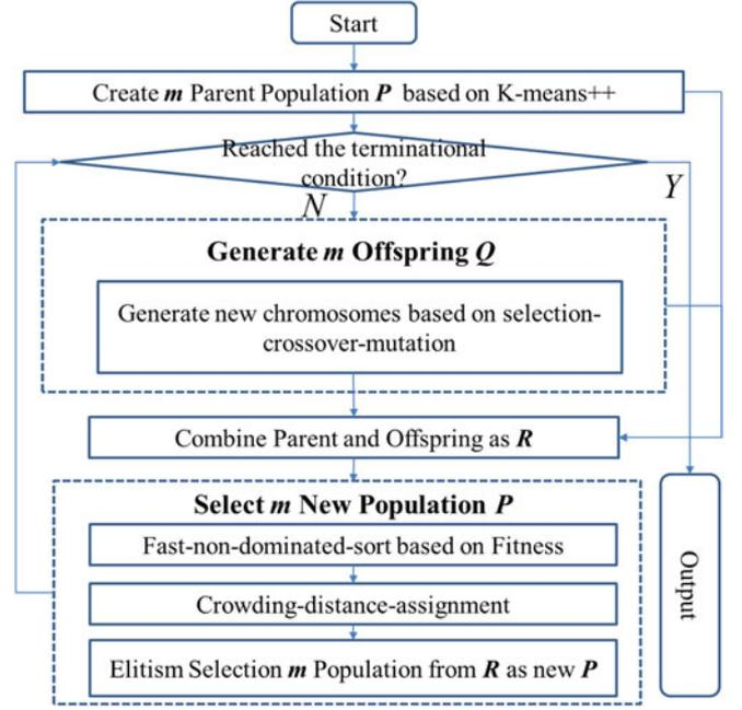
Fig. 5. Flowchart for cluster optimization using NSGA-II.
