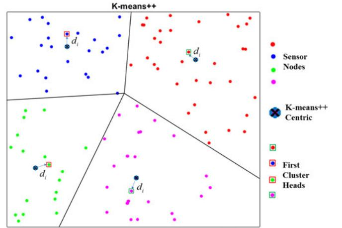
Fig. 4. Cluster initialization based on K-means++.
