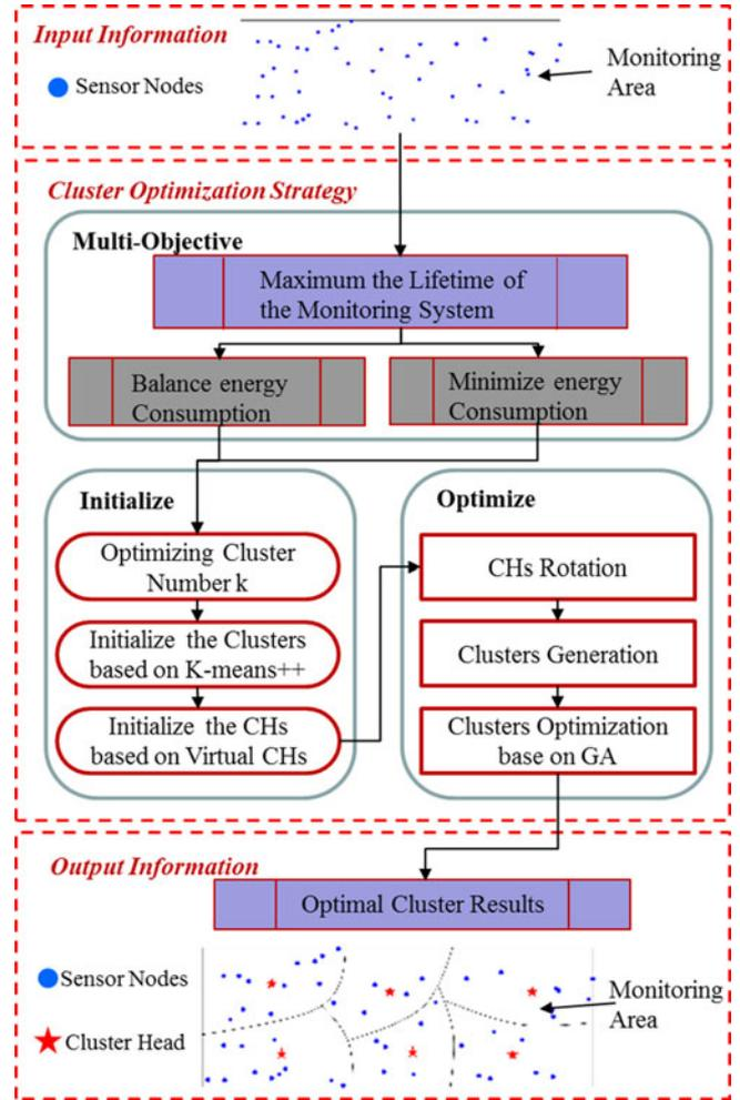
Fig. 2. Overall scheme of RIWMS sensor cluster optimization.
