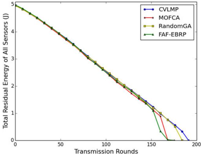
Fig. 8. Comparison of the total residual energy of all sensors.
