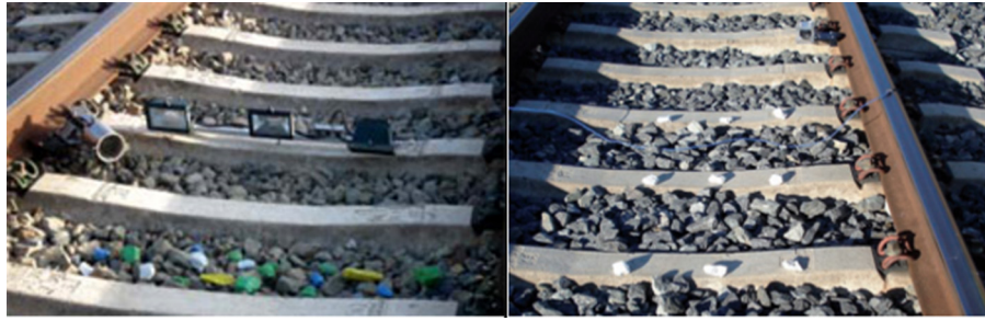
Fig. 8. HSR site test of ballast flight [52].
